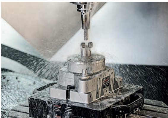
MANOK plus manual stationary chuck in use
