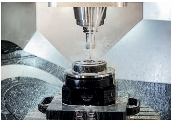
HYDROK hydraulic stationary chuck in use
